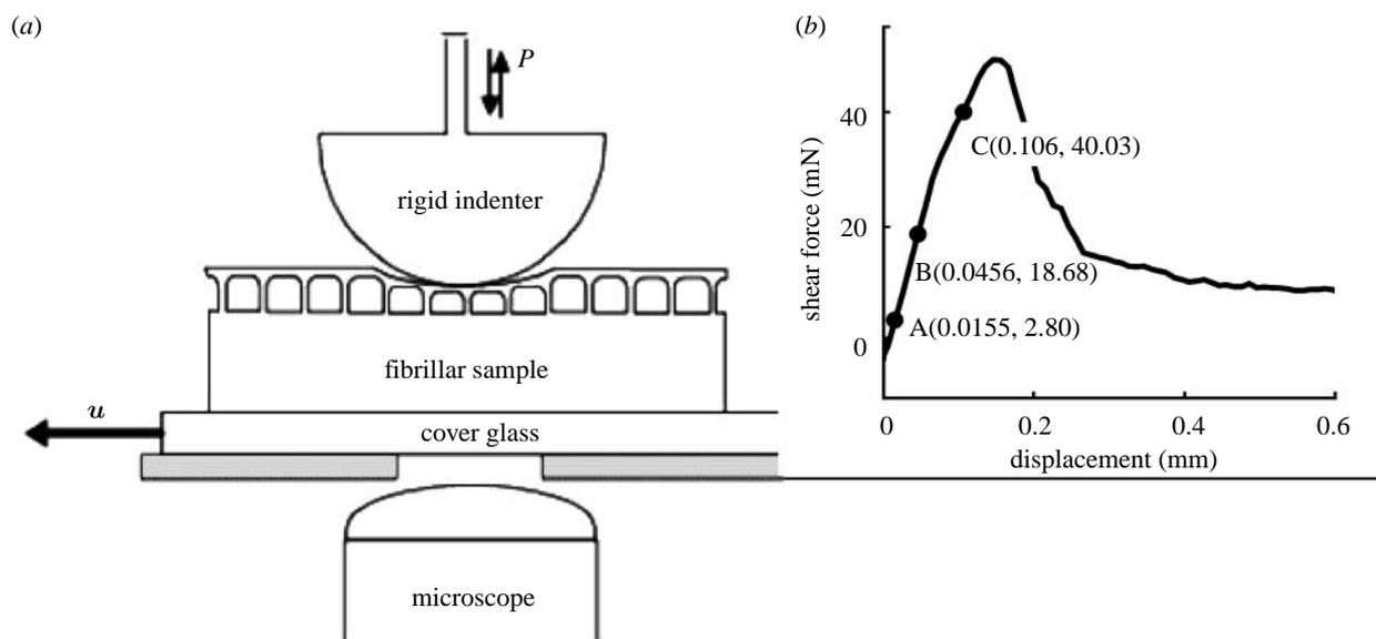
Figure 1. (a) A glass spherical indenter is placed on the surface of a microfibril array under a fixed normal force ( $P$ ) (applied via a mechanical balance). The sample is translated at a constant rate,  $u$ , and the shear force is measured by a load cell. Deformation near the contact region is recorded by means of an inverted optical microscope. The shear load versus shear displacement curve for a fibrillar sample is shown in (b). Three points are selected for comparison with the theory.
