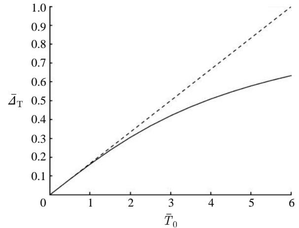
Figure 5. Normalized shear displacement,  $\bar{\Delta}_T$ , versus normalized shear force,  $\bar{T}_0$ , for  $\bar{N}_0 = 0$  (or  $\theta_0 = 0$ ) and  $b/L_0 = 14/67$ . Solid line, the solution of the nonlinear theory (2.28)–(2.30); dashed line, the prediction of BCM (2.31).
