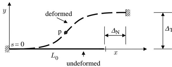
Figure 3. The coordinate system used in our analysis. The undeformed beam is straight and has length  $L_0$ . Both the ends of the beam are clamped. The right end is subjected to a vertical and tangential displacement  $\Delta_N$  and  $\Delta_T$ , respectively. The coordinates of the point 'p' are  $(x(s), y(s))$ .
