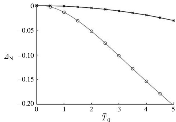
Figure 7. The normalized normal displacement,  $\bar{\Delta}_N$ , versus normalized shear force  $\bar{T}_0$ , for  $\bar{N}_0 = 0$  (or  $\theta_0 = 0$ ). It shows that a significant normal deflection at the fibril end can occur with no applied normal force. Note that the small-deflection theory underestimates the normal displacement. Circles, large-deflection theory; crosses, small-deflection BCM.
