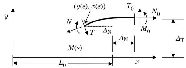
Figure 4. The free-body diagram of a section of the deformed bar. The right end of this section is clamped ( $\psi=0$ ).  $\Delta_T$  and  $\Delta_N$  are the shear and normal displacements, respectively, at the right end of the beam.  $N_0$  and  $T_0$  denote the reaction forces, whereas the reaction moment is denoted by  $M_0$ .
