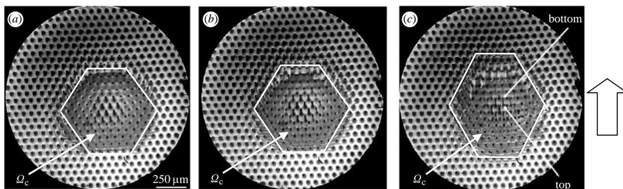
Figure 2. Optical micrographs of the contact region. The direction of shear displacement  $u$  is indicated by the arrow on the right. The image of the top end of a fibril appears as a fuzzy grey circle, whereas the bottom end appears as a smaller dark square. This difference allows us to determine the relative deflection  $\Delta_T$  of each fibril. (a–c) correspond to the points A–C in figure 1b, respectively. The contact region  $\Omega_c$  is the white polygon.
