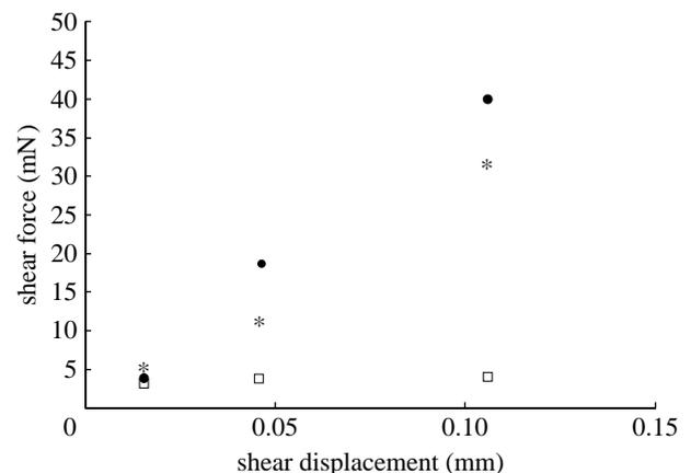
Figure 10. Comparison of the experimental data (stage 1, filled circles) with the large- (asterisks) and small- (squares) deflection theoretical results. The small-deflection theory (BCM) works well for very small shear displacements but considerably underestimates the shear force for large shear displacements.
