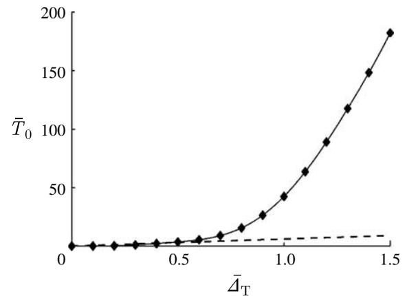
Figure 9. Normalized shear force versus normalized shear displacement for  $N_0 = 0$ . The dashed line is the small-deflection BCM (2.31). The seventh-order polynomial fit (3.1) (solid line) captures the numerical result (diamonds) obtained by solving (2.28)–(2.30). Normal compression is assumed to be zero.
