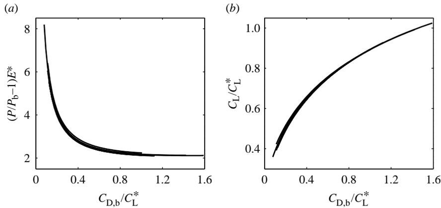
Figure 2. Minimal power required for (a) swimming and (b) the associated lift coefficient.  $C_{D,0}$  varies between 0.008 and 0.02 (about twice its maximal expected value), and  $k$  varies between 0.05 and 0.1. (a, b) All feasible combinations of these parameters result in practically indistinguishable differences.
