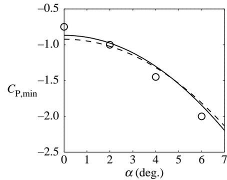
Figure 7. Minimal pressure coefficient on the surface of a 0.2 chord thick dolphin caudal fin. Circles mark the data extracted from fig. 2 of Lang (1966), dashed line marks the approximation (A 12) with  $t=0.2c$  and solid line marks the approximation (A 14) with  $r_{LE}=0.042c$ .
