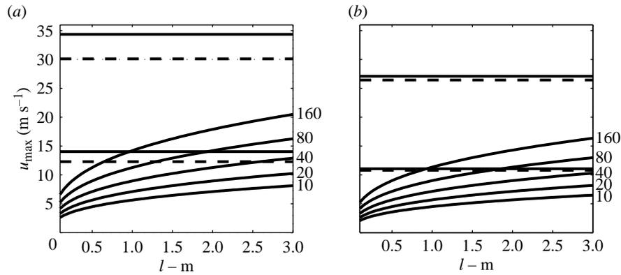
Figure 6. Maximal swimming velocity with  $\bar{h} = 0.2$ ,  $C_{D,0} = 0.01$ ,  $k = 0.05$ ,  $C_{L,max} = 1.2$ , (a)  $C_{D,b} = 0.2$  and (b)  $C_{D,b} = 0.4$ . Curved solid lines mark power limit on the swimming velocity—the respective power per unit mass of the fish is marked to the right of each line. The horizontal lines mark cavitation limits for 9% (solid lines) and 20% (dashed lines) thick foils near the surface (lower sets) and at the depth of 50 m (higher sets).
