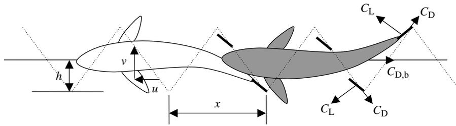
Figure 1. Swimming model. With fish body moving along the solid horizontal line, the tail is assumed to move along the dotted sawtooth trajectory. Its wave-length,  $x$ , is the stride length and its depth is  $2h$ . The ratio of  $4h$  and  $x$  is also the ratio of the (presumably constant) lateral tail velocity  $v$  to the (constant) swimming velocity  $u$ .
