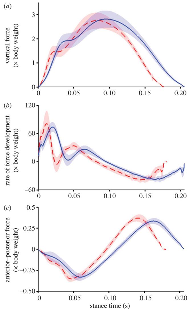
**Figure 3.** Group mean  $\pm$  s.d. (shaded area) for vertical force (*a*), vertical force loading rate (*b*) and anteroposterior force (*c*). Data are recorded from each participant running barefoot (red) and shod (blue) at  $3.89 \text{ ms}^{-1}$  and presented from foot contact to toe-off from the right foot. Loading rate is defined as the first derivative of the vertical ground reaction force signal. All data are normalized to body weight. (Online version in colour.)
