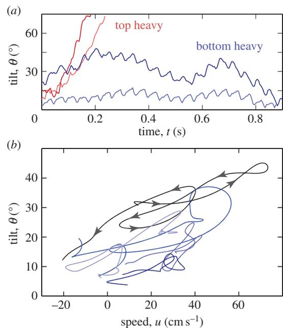
**Figure 5.** Stability during hovering. (a) Typical tilt dynamics measured from high-speed video. The flyer has a low centre of mass (bottom heavy) and undergoes stable oscillations. An earlier prototype with a motor attached high on the body (top heavy) flips over in a few wing-beats. (b) Tilt is correlated with horizontal speed for five hovering sequences. Excursions to high tilt are accompanied by high speed, causing the flyer to return to low angle. (Online version in colour.)
