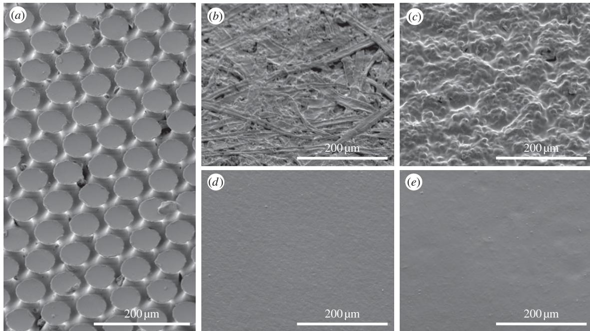
**Figure 1.** Mushroom-shaped adhesive microstructure made of (a) PVS and Epoxy counterfaces (b) 6, (c) 4, (d) 1, (e) 5, with numbers according to table 1.
