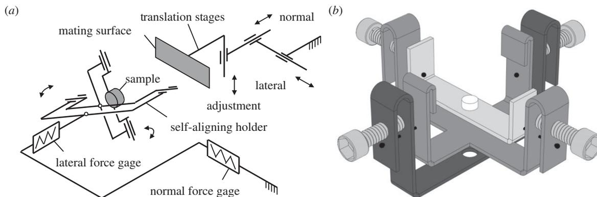
**Figure 2.** (a) Schematic of the home-made tribometer used [27]. (b) Passive self-aligning sample holder based on two orthogonal axes of rotation coplanar with the contact plane [27]. The system is made much more user-friendly by using thread-tightening screws simplifying considerably preliminary adjustments.
